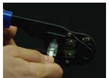
**9** Then we introduce the wires inside the connector watching that they enter their lane until they make a stop with the bottom.
