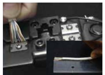
**5** When it is cut, strip the insulation until you see the 8 threads crossed in 4 pairs.
